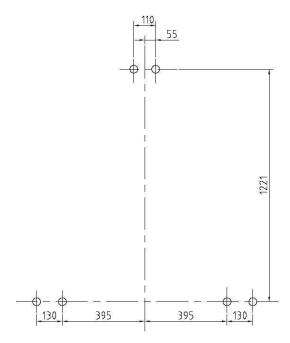
(85-inch Board layout for installation)
